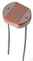
Gambar 2. 5 Light Dependent Resistor
