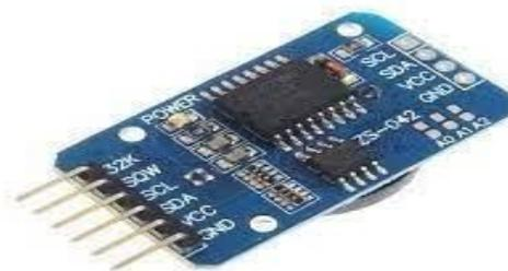
Gambar 2. 7. Real Time Clock (RTC)
