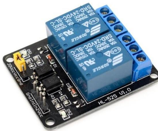
Gambar 2.7 Relay 2 Channel
