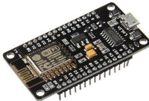
**Gambar 2.2.** ESP 8266 NODEMCU V3
