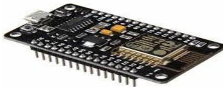
Gambar 2. 1 NodeMCU ESP8266 Devkit
