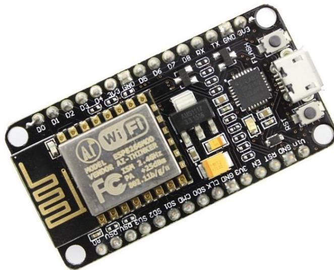
**Gambar 2.2. NodeMCU Lua WIFI Board Based on ESP8266 CP2102**
