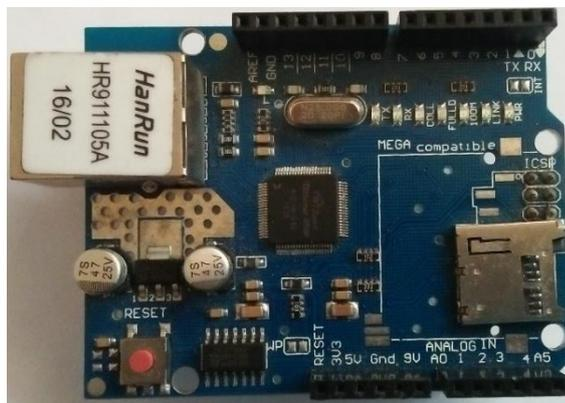
Gambar 2.7. *Ethernet Shield*
