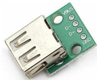
*Gambar 2.11 Female USB Type A to DIP 2.54mm Adapter*
