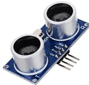
Gambar 2.4 Sensor Ultrasonic
