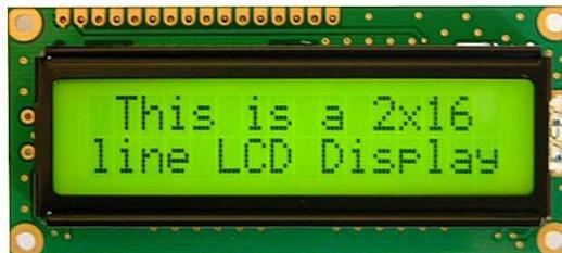
Gambar 2. 11 LCD Crystal Display 16x2
