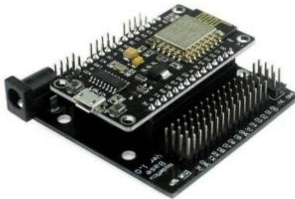
Gambar 2. 3 Board NodeMCU
