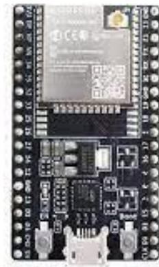
Gambar 2. 1 Modul ESP32 DEVKITC V4
