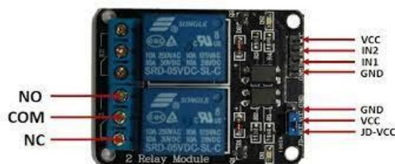
Gambar 2. 3 Pin Relay 2 channel
