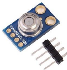
Gambar 2. 9 Sensor Infrared MLX 90614
